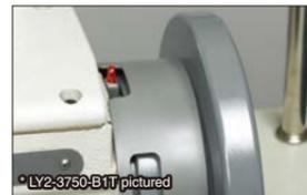
Upper and lower needle stop positions can be separately adjusted with a single operation. The display lamp shows the power status at a single glance. (Supports LY2-3750/LY2-3310/LY3-6840)
