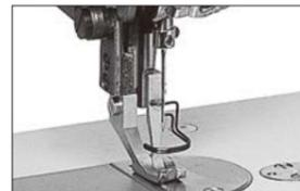
Uses vertical feed to clamp and reliably feed material that is difficult to feed.
