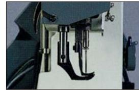
After thread cutting, the reverse function of the sewing machine can be used to prevent the needle from coming out from the holder and to ensure the holder is raised to 16mm. This function ensures easy insertion and removal of thick materials.
