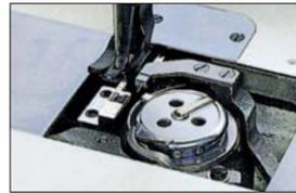
The meshing of the fixed female and the female linearly moving in parallel with the feed dog enables excellent cutting of thread from fine to thick threads (#8).
