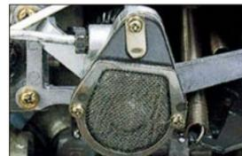
An automatic oil lubrication system eliminates the need to feed oil. Oil in the oil tank is supplied by pump to required areas, thereby improving durability of the sewing machine. (Supports LY2-3750/LY3-6840)
