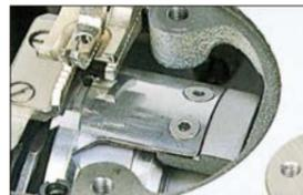
Our proven left female rotating and right female fixed meshing system enables excellent cutting of thread from fine to thick threads (#6). (Supports LY2-3750/LY2-3310)
