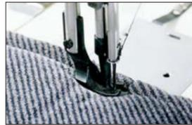
The lineup includes a CS-specification model for sewing car seats and other projects. Changes have been made to the balance stroke and feed motion to further improve sewing quality in seat sewing projects.
