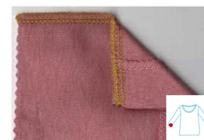
Four threads back latching stitch
