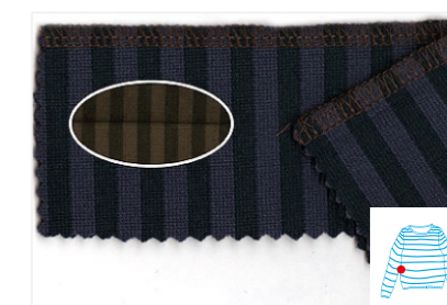
Four threads variable top feed
