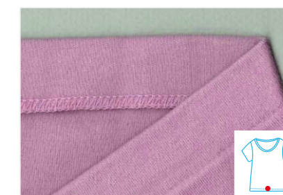
Three threads blindstitch hemming
