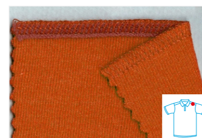
Four thread tape attach stitch
