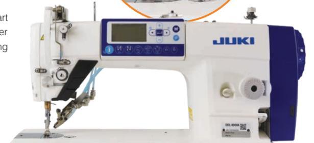
Sample installation of bird's nest prevention device
