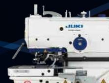
Computer-controlled, Eyelet Buttonholing Sewing System (Trimmer for Needle and Loper Thread with gimp)
