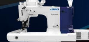
High-speed, Feed-off-the-arm, 3-needle Double Chainstitch Sewing System (Digital workstation)
