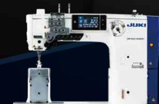
Semi-dry Direct-drive, Post-bed, Unison-feed, Lockstitch Sewing System with Vertical-axis Large Hook
