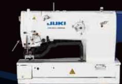
Computer-controlled, High-speed, Buttonholing Sewing System
